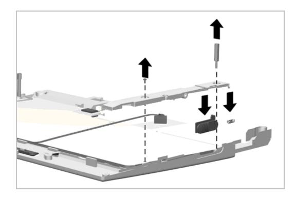
Figure 5-45. Removing the MultiBay Release Assembly
